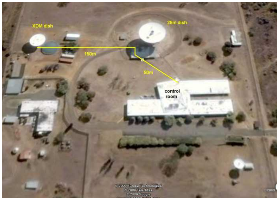
Figure 3.5: Picture of HartRAO radio observatory and XDM dish with optical cable path (as adapted from [8])
